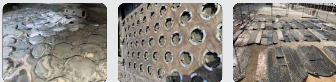
Figure : Condition of U-26 TR-2 Deposit Trays - Before & After Cleaning
